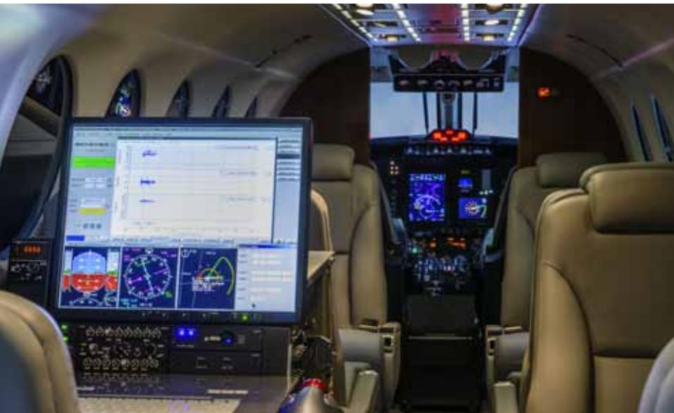
Flight inspection systems by Aerodata
